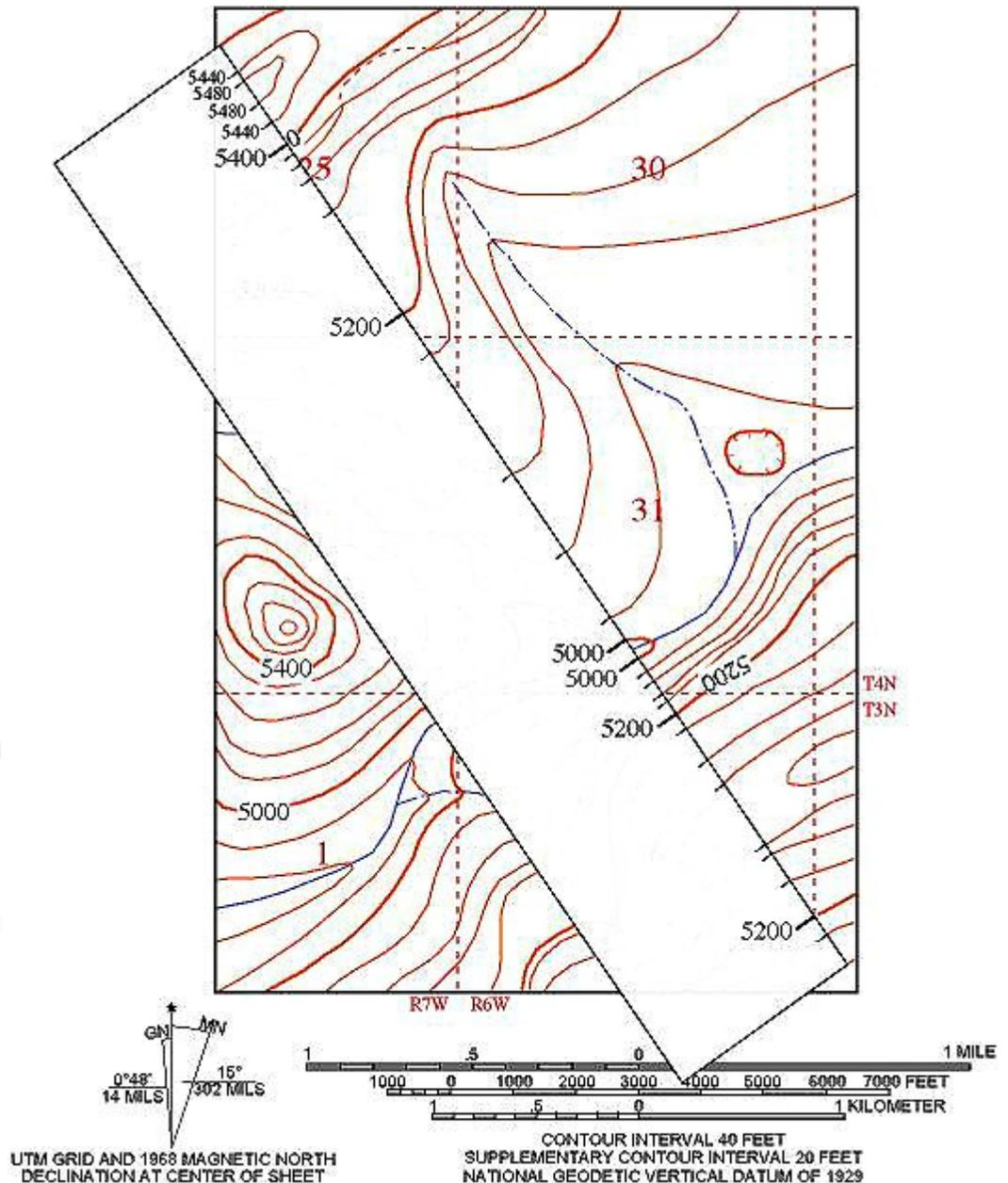
3) On both the blank paper and the map (or mylar), mark clearly the starting and ending points of your line of section. Below these marks, write down the elevation of the starting and ending points of your section.
