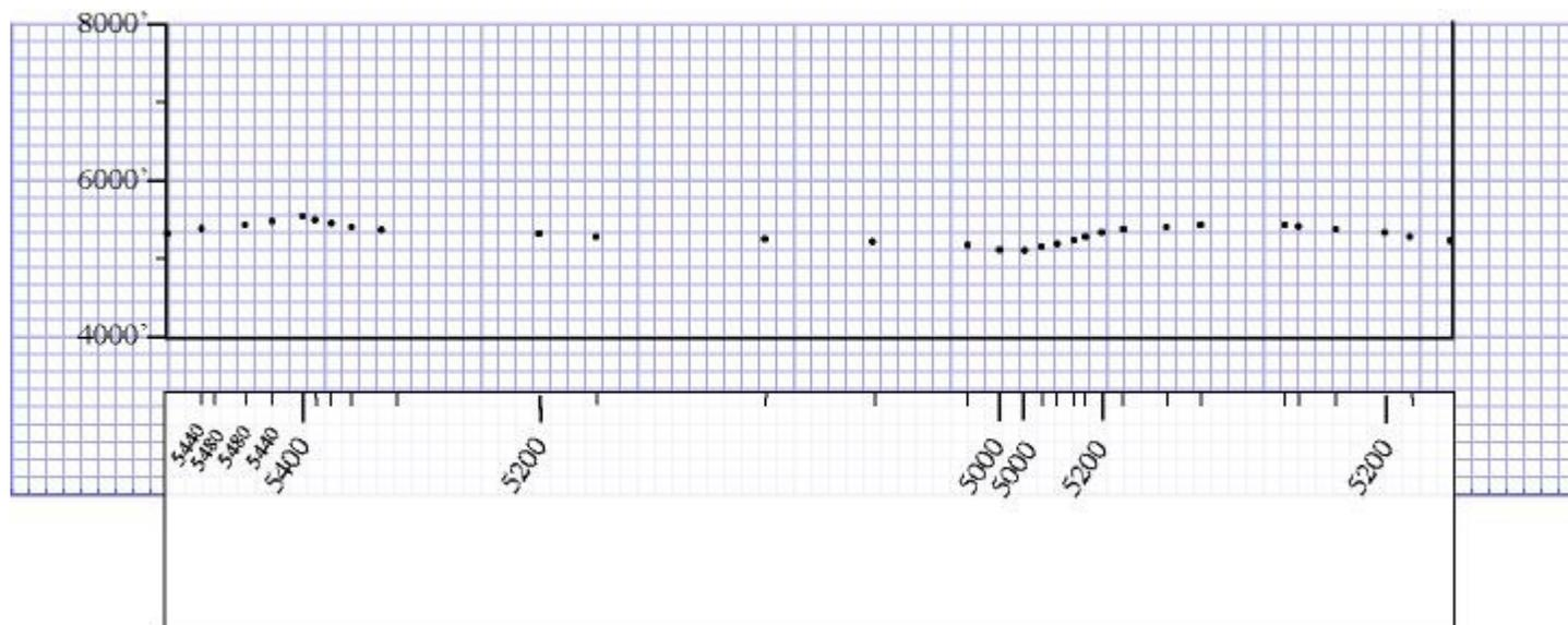
8) Connect the dots on the graph paper, and you have a topographic profile.
