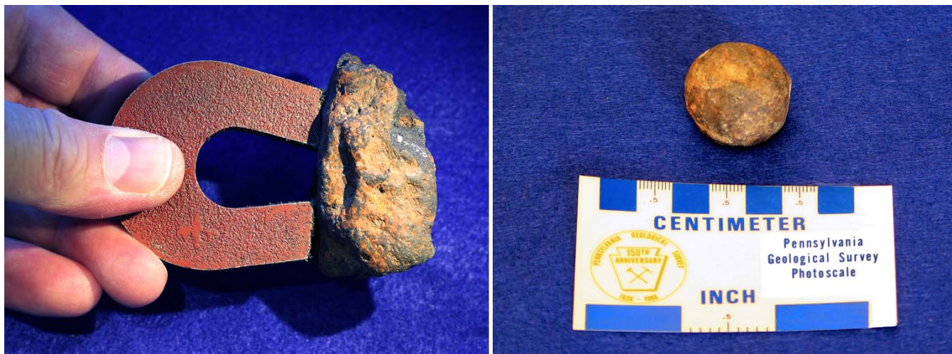
Figure 16. Two of many samples brought to the Pennsylvania Geological Survey because they were thought to be meteorites. The sample on the left is likely the result of an industrial process (iron slag) and contains enough iron to stick to a magnet. The sample on the right is canister or grapeshot (location unknown), perhaps from the Revolutionary War or Civil War.
