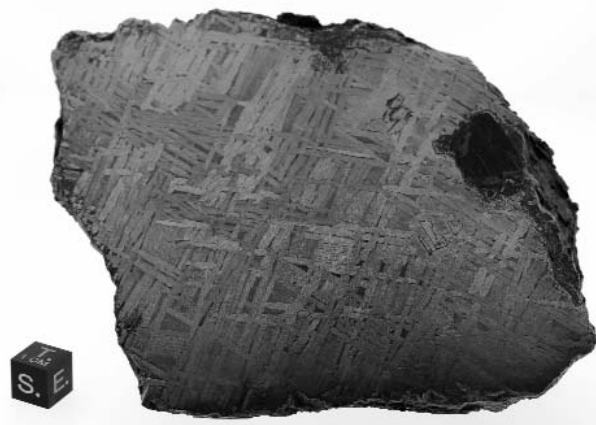
Figure 12. Detailed slice of the Shrewsbury meteorite, discovered in 1907 in Shrewsbury, York County, Pa. Note the complex interlocking pattern of iron-nickel bands, or Widmanstätten pattern. Natural History Museum, Vienna, specimen Shrewsbury_J2286_LF1. Photograph by Ludovic Ferrière, Natural History Museum, Vienna, Austria.
