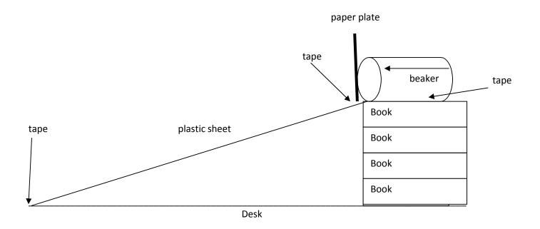
9. When you are ready to begin, lift up the paper plate to allow the glop to flow/creep down the sheeting. At thirty seconds increments, take a measurement of how far the glop has moved. 0 cm is the edge of the beaker. Read the increments that you have already marked on the sheeting. Record your data in the table below. Keep recording for the full 10 minutes. It is OK to slightly tilt the beaker to get a flow started. If needed, make a new mixture and start again.
